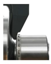
5. Use the SKF mounting tool VKN 600 to fit the bearing.
