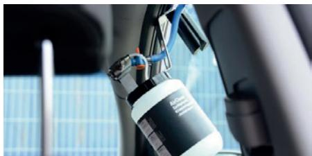
7. Set the fan to the medium setting at approx. 20°C, open all air nozzles and set the ventilation to circulation mode. Set up an external power supply for the vehicle electrical system or leave the engine running.
