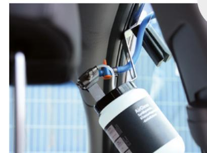
Set up an external power supply for the vehicle electrical system or leave the engine running. Close the doors and leave the door that the ventilation supply hose is fed through propped open in order to prevent too much of the mist from escaping. Open the compressed air supply and let the disinfectant flow in until an obvious saturation/formation of mist is visible inside the vehicle.
