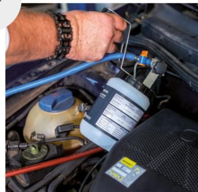
5. Open the bonnet and remove the cabin filter. Clean the pollen filter box if required and disinfect it. Set the ventilation system to level 1 and spray the disinfectant into the interior of the vehicle through the air intake opening of the HVAC system. Feed the agent in until the vehicle interior has become visibly filled with mist. Leave the mist to take effect for approx. 1 minute.
