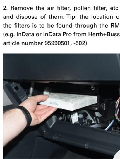
2. Remove the air filter, pollen filter, etc., and dispose of them. Tip: the location of the filters is to be found through the RMI (e.g. InData or InData Pro from Herth+Buss, article number 95990501, -502)
