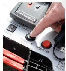
4. Then use the "Test case ON" switch to start the testing process.
