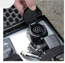
2. The socket integrated in the trailer test case allows both 7- and 13-pin 12V trailer cables to be connected.
