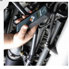
You can read out the respective hydrogen concentration on the display. Rising ppm values indicate a leak.
