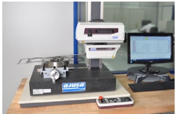
Therefore, it is necessary to have a contact measurement where precision under a micron makes this tool vital for both the design and the verification of the products.
