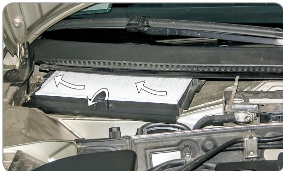
EN Remove the filter lock. Remove the old filter from the seat, put the new one in and perform the opposite to all the previous actions in the reversed order
