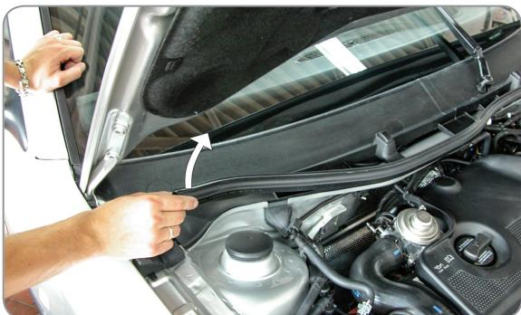
EN Remove the rubber seal
